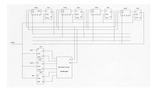
SINCE DATA MUST REMAIN IN THE SAME ORDER (BUT ROTATED) IO = FUP-FOP OUTPUT I, = ONE FF TO THE RIGHT IZ = TWO FF TO THE RIGHT I3 = THREE FF TO RIGHT (ORDER TO THE LEFT ALSO WORKS)
