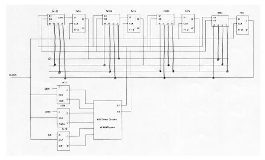
2. The count and direction inputs are applied to the MUX select circuitry via 7474 D flip flops, hence both the true and complemented versions will be available (inverters not required). Based on the connections defined in part 1, design the MUX select circuitry using only NAND gates. Include Karnaugh maps and the minimized Boolean equations; you do not have to draw the schematic.
