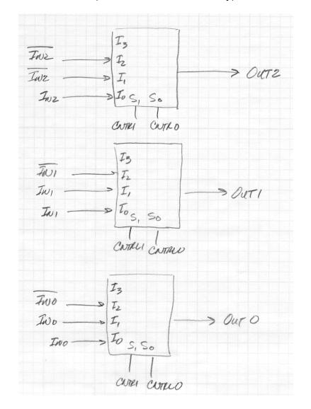
3. Adding three full adders and a single AND gate to the design in part 2, complete the design to generate the 2's complement of the number (Cntrl1, Cntrl0 = 11).
